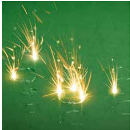
Dental frameworks being made by the additive manufacturing process of laser melting © Renishaw
